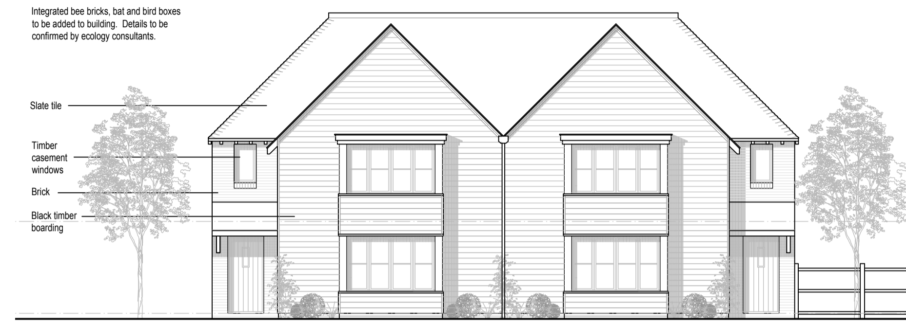
Proposed South West Elevation Scale 1:100
